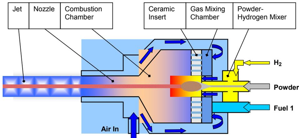
Figure 1: Schematics of HVOF gun
