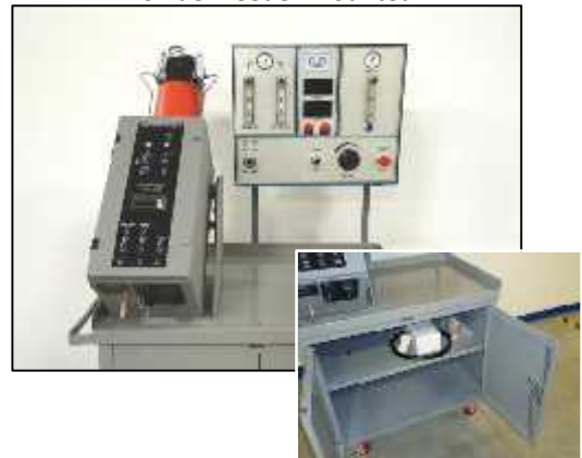
Mobile Cart with Control Console and Powder Feeder Mounted
