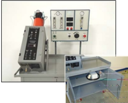
Mobile cart with Control console and Powder Feeder Mounted
